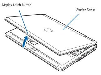
Figure 3-2. Opening the Display Panel
